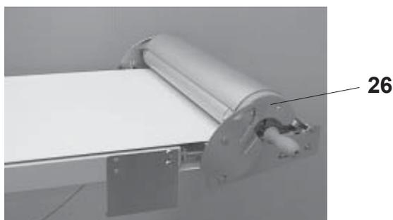
Working position of the automatic reeler unit (closed)
